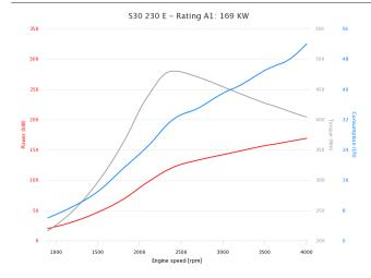
$^{\star}$  Net Power at flywheel according to ISO 8665, after 50 hours running, Fuel Diesel EN 590. Power tolerance 5%.
